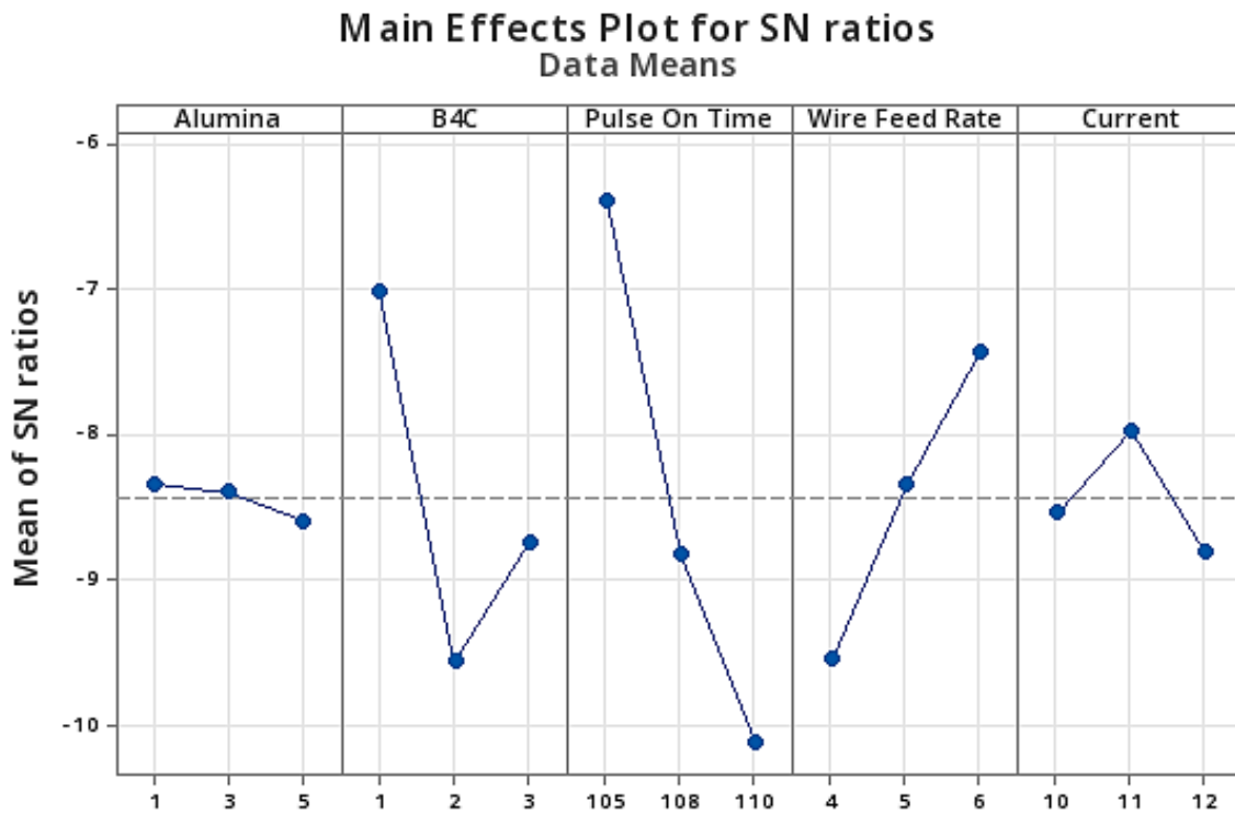
Figure 2. Effect of Input Parameter on Surface Roughness by Plot SN ratios.
