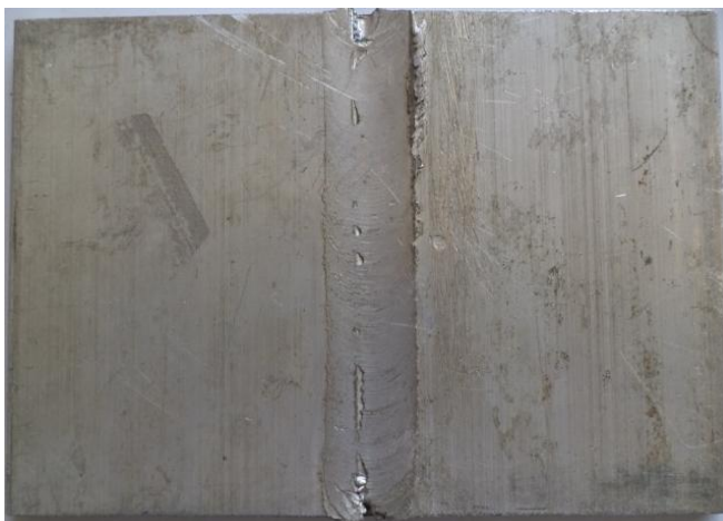
Figure 7. Improved condition of weldment Al 8010 sample.
