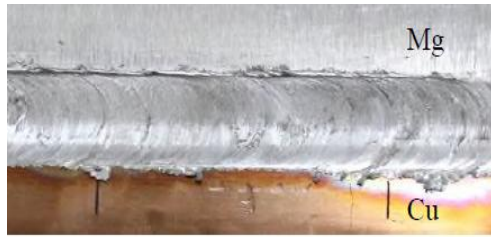
Figure 6 (a). Surface appearance Copper to Mg [29]
