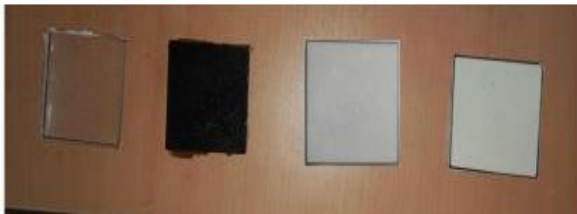
Figure 1. Pure resin, Fe 2 O 3 , ZnO and MgO polymeric composite sheets.
