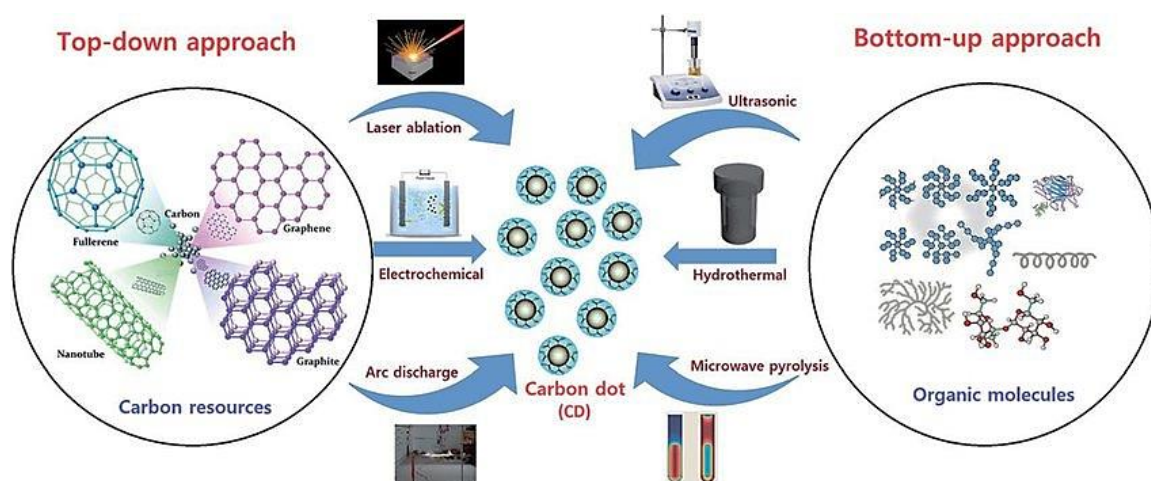
Figure 7. Synthesis methods to prepare carbon dots.
