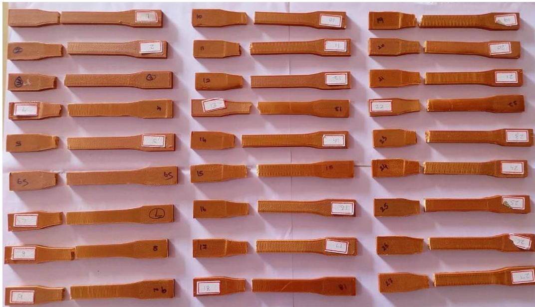
Figure 4. Specimens after tensile testing.
