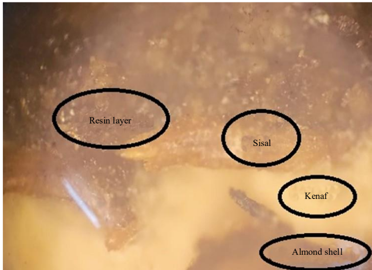
Figure 7. Microscopic image of kenaf: sisal: almond shell: epoxy (25%: 25%: 15%: 35%).
