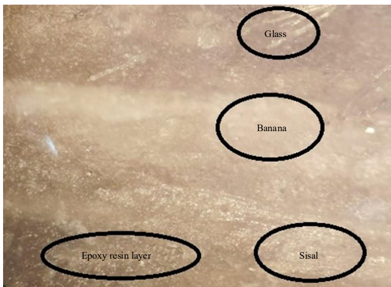
Figure 8. Microscopic image of banana: sisal: glass: epoxy (25%: 25%: 20%: 30%).
