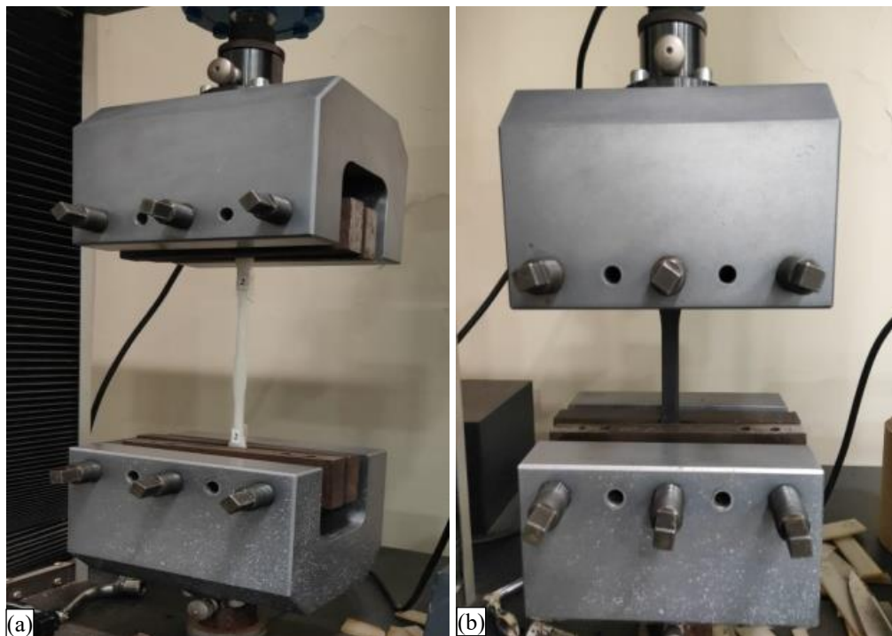
Figure 4. Tensile testing of specimens: (a) nylon and (b) polyethylene terephthalate glycol (PETG).
