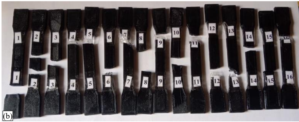
Figure 5. Tested specimens: (a) nylon and (b) polyethylene terephthalate glycol (PETG).
