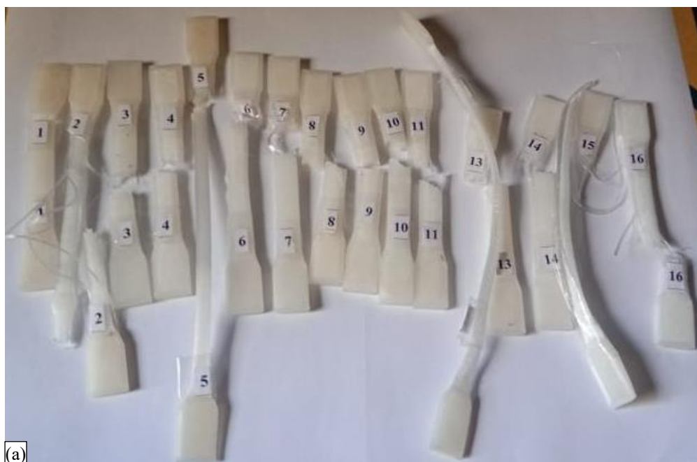
Figure 4. Tensile testing of specimens: (a) nylon and (b) polyethylene terephthalate glycol (PETG).
