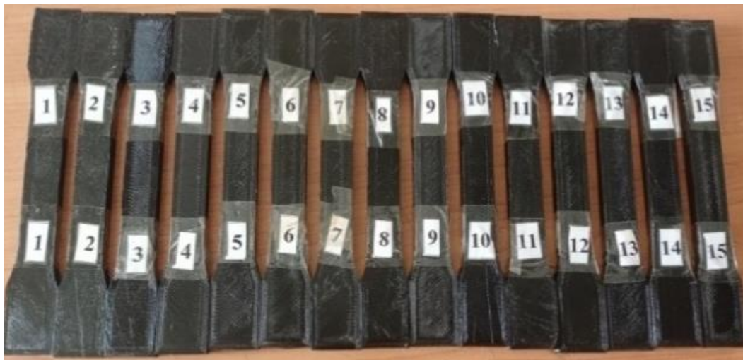
Figure 3. 3D printed specimens of polyethylene terephthalate glycol (PETG).
