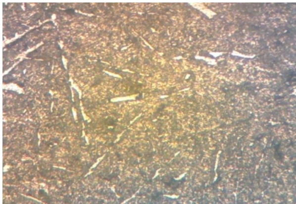
Figure 1. Microstructure of sample 'A' at 200X magnifications.
