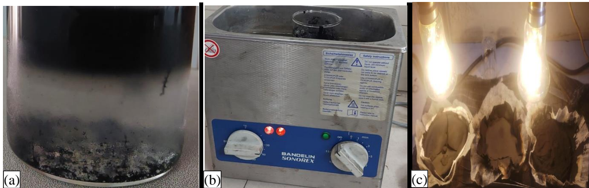
Figure 2. (a) Synthesis of graphene oxide through Electrochemical method, (b) Sonication process of graphene oxide using Bath sonicator, (c) Drying of graphene oxide after exfoliation process.
