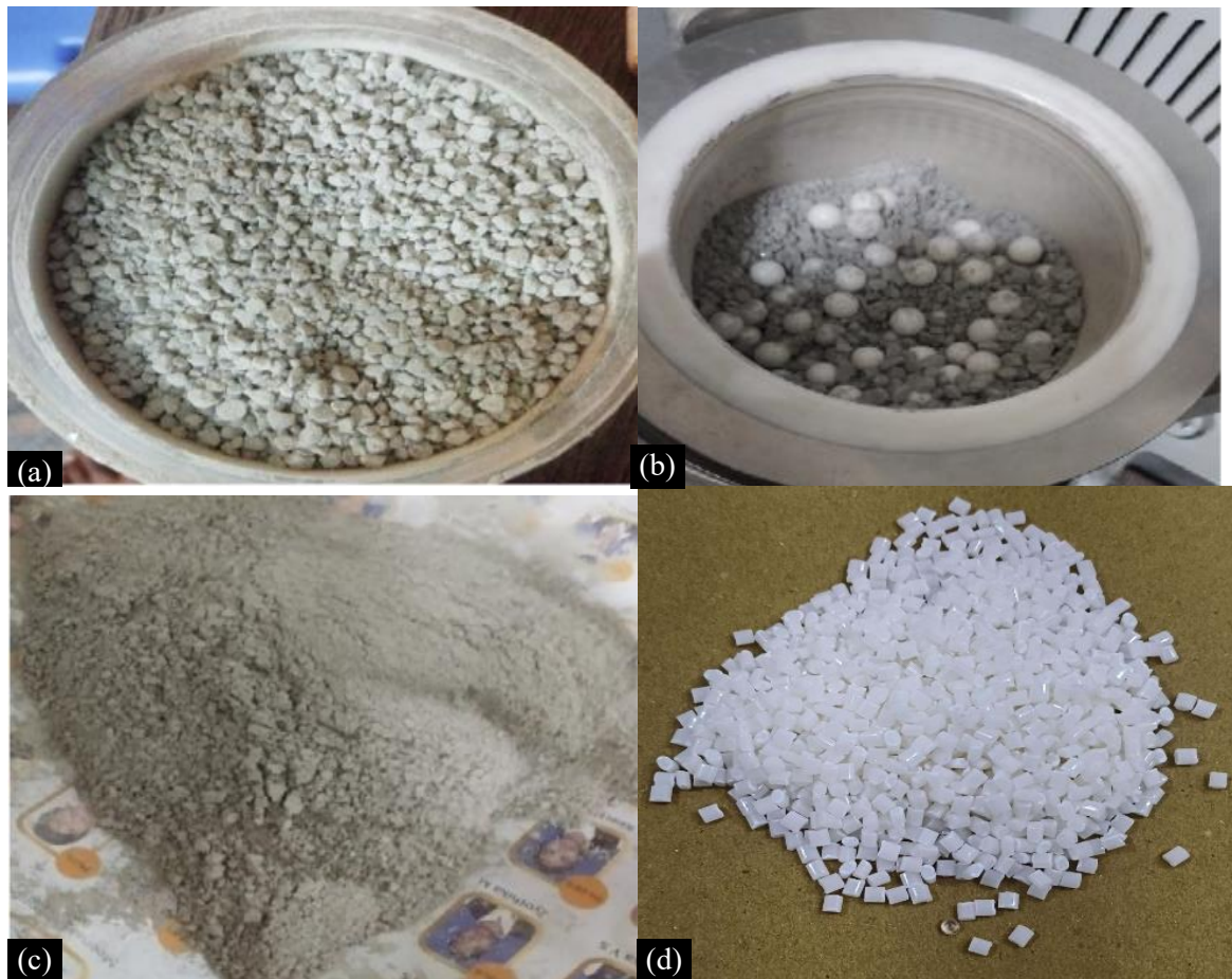
Figure 1. Production Process of Epoxy Micro Particles from Rectangular Blocks. a - Shows Epoxy Granules Obtained by Breaking Rectangular Blocks, b - Shows Ball Milling of Epoxy Granules, c – Shows Cross Linked Epoxy Micro Particles and d - Shows Natural ABS Polymer Pellets.
