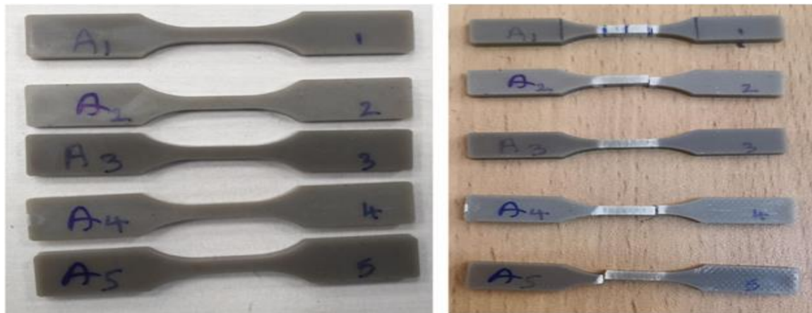
Figure 3: Tensile Testing Specimens A1 (100%ABS + 0%E), A2 (95%ABS + 5%E), A3 (90%ABS + 10%E), A4 (85%ABS + 15%E) and A5 (80%ABS + 20%E) Before and After Testing.
