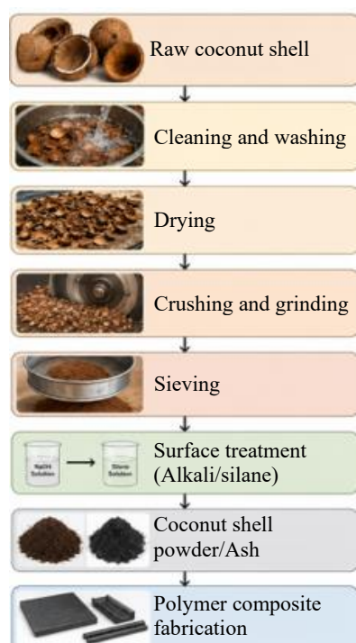
Figure 1. Processing route for coconut shell fillers used in hybrid polymer composites.
