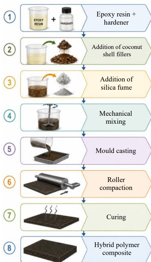
Figure 3. Hand lay-up fabrication process for hybrid polymer composites.
