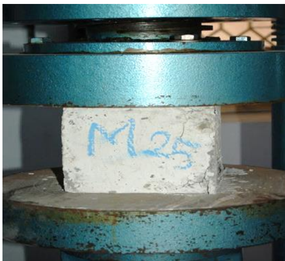
Figure 3. Failure pattern of cube under compression.
