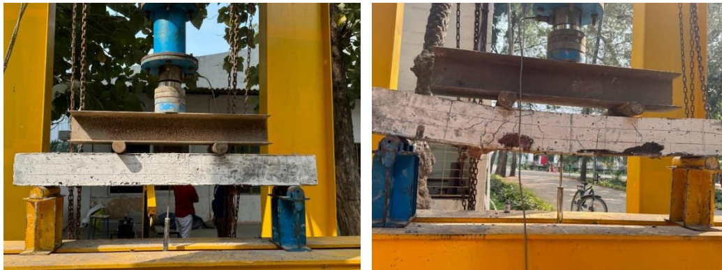
Figure 23. Beam testing for Replacement of POFA and OPC.
