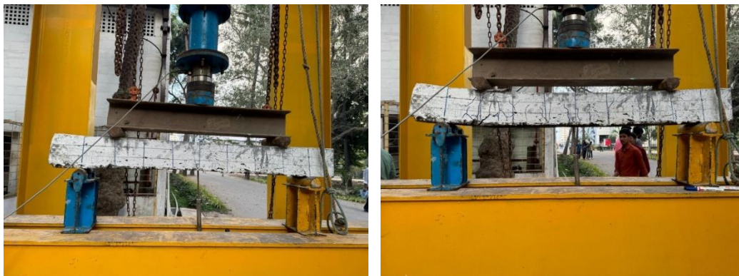
Figure 22. Beam testing for Conventional concrete.
