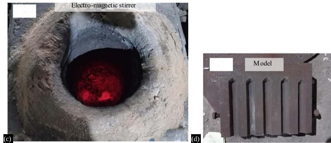
Figure1. Stir casting setup and study materials (a) melting of Al319 using furnace, (b) SiC and GNPs reinforcement particles, (c) electro-magnetic stirrer, and (d) mold for samples.
