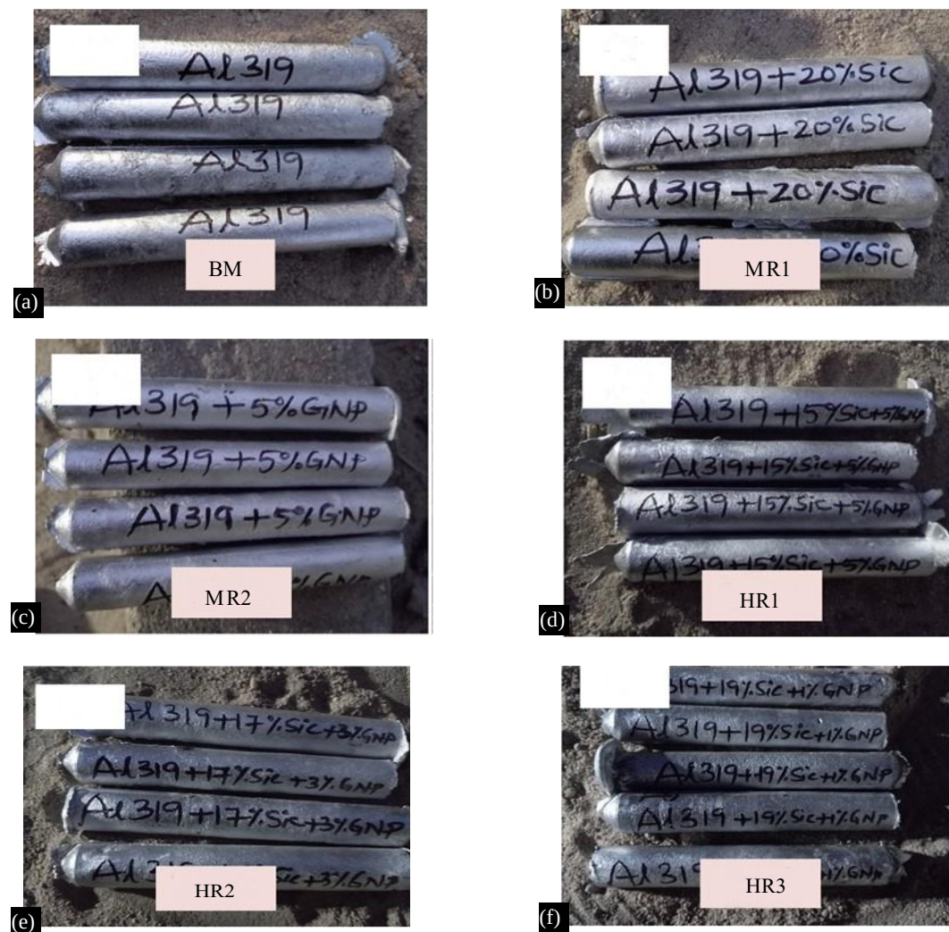
Figure 2. Fabricated study composite samples (a) BM, (b) MR1, (c) MR2, (d) HR1, (e) HR2, and (f) HR3.
