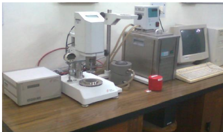
Figure 3. Rheometer (Physica MC1) for rheology measurement.
