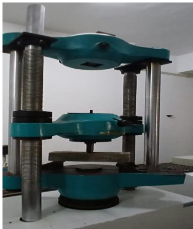
Figure 5. (a) – Arrangement of universal testing machine with prism centred for loading.
