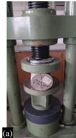
Figure 4. (a) – Split Tensile Strength on M30 Concrete Mix Cylindrical Specimen
