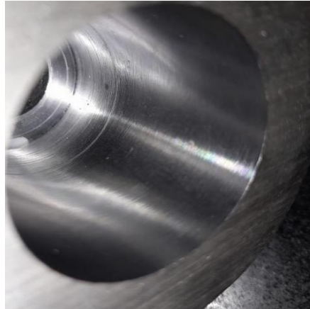
Figure 10. Chatter free machined surface with modified tool.
