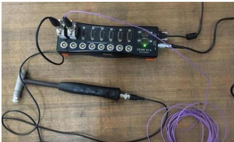
Figure 2. Impact hammer and 8 channel data acquisition (DAQ) system.
