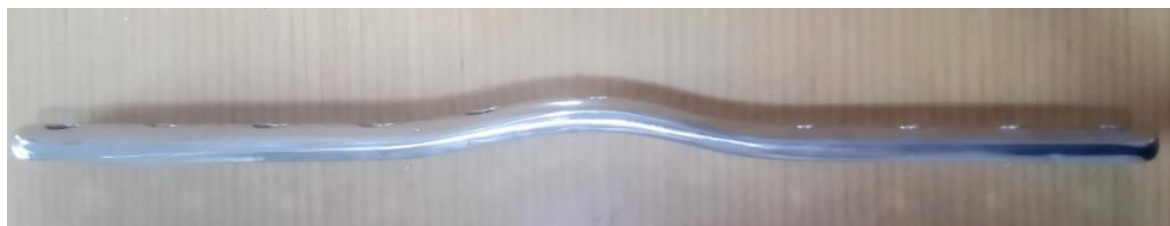
Figure 26. The wave plate with 15° of central curved segment.
