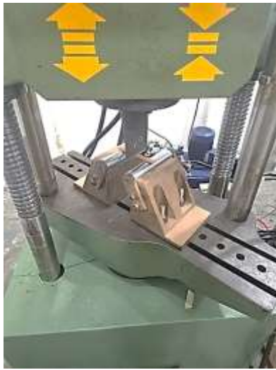
Figure 4. 3-point bending test of specimen.
