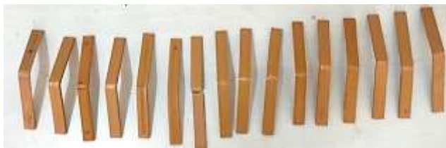
Figure 5. Flexural specimens after testing.
