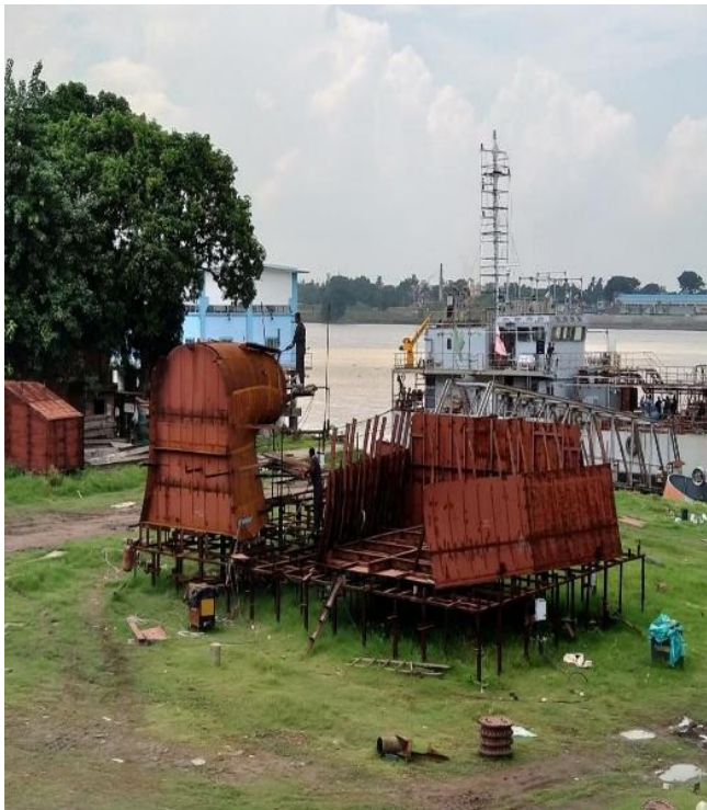
Figure 8. Ship Bulbous welding.
