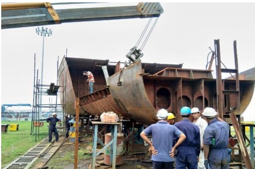
Figure 12. Y-283 Plate cutting work in progress.
