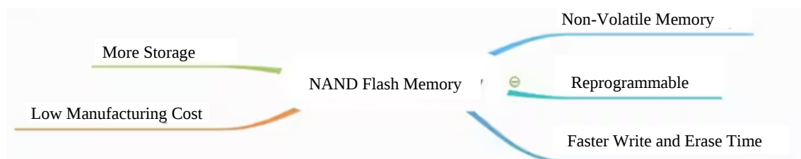
Figure 6. Features of NAND flash memory.
