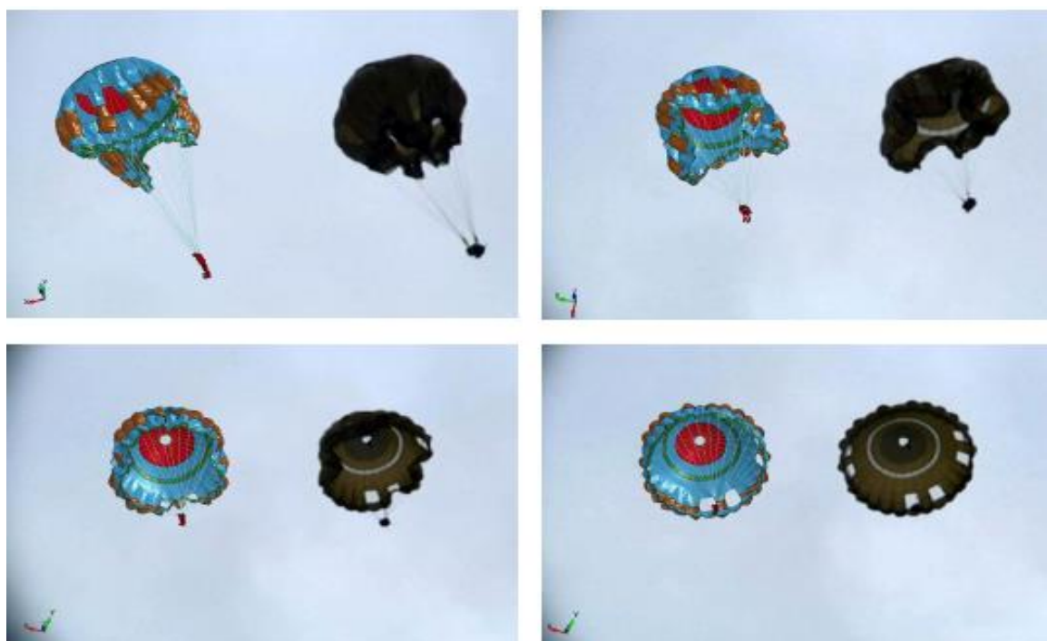
Figure 13. Real and computed profiles compared at different times during the opening.
