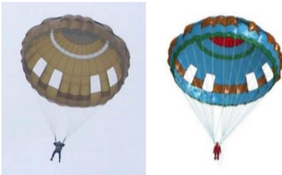
Figure 4. Real and simulated inflated profiles of the EPC.
