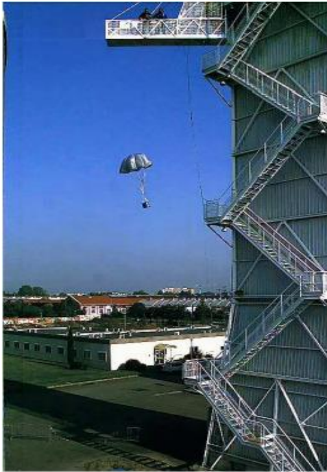
Figure 9. Drop of a small hemispherical parachute.
