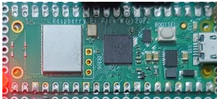
Figure 2. Raspberry Pi Pico W microcontroller used as the central processing and control unit in the proposed system.
