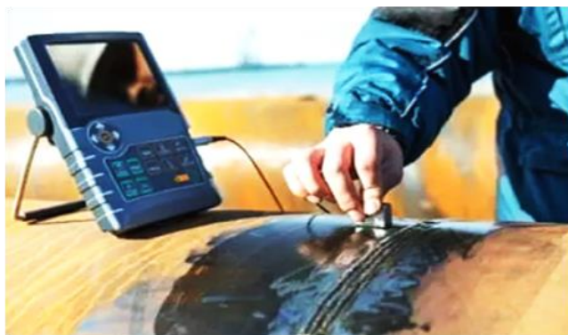
Figure 10. Thickness checking with an ultrasonic thickness gauge.
