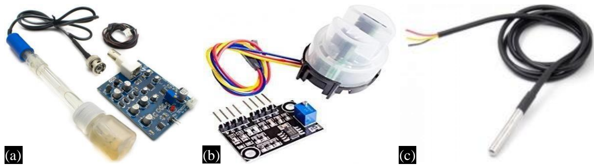
Figure 4. Sensors utilized: (a) pH sensor, (b) turbidity sensor, (c) temperature sensor.
