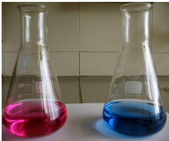
Figure 3. Estimation of total hardness by EDTA method.
