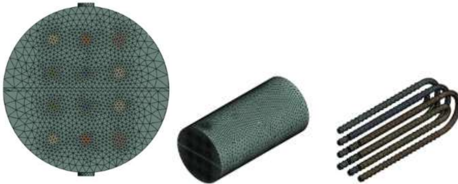
Figure 2. Mesh analysis of corrugated U-tube shell and tube heat exchanger.
