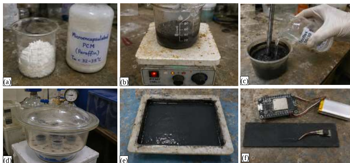
Figure 1. Fabrication process of stretchable elastomer–PCM composite and wearable IoT temperature monitoring device. (a) Microencapsulated paraffin PCM material, (b) Dispersion of PCM with conductive fillers, (c) Addition of silicone elastomer and mixing, (d) Vacuum degassing of composite slurry, (e) Casting and curing of composite sheet, (f) Final wearable device with BLE temperature sensor integration.
