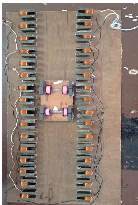
Figure 2. Electromagnetic propulsion train.
