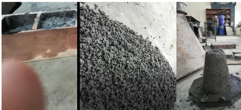
Figure 2. GPCC during the slump test and casting of cubes using a table vibrator.
