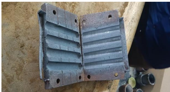
Figure 3. Graphite Coated moulds and casted samples in the dies.
