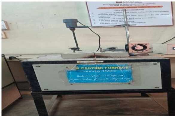
Figure 2. Stir Casting Setup & Crucible
