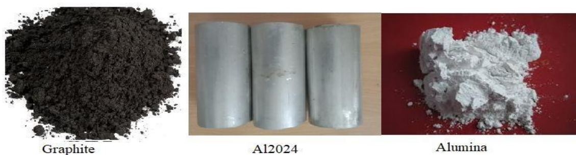
Figure 1. Matrix and reinforcements used in synthesis of monolithic and hybrid composites.
