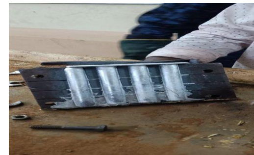
Figure 3. Graphite Coated moulds and casted samples in the dies.
