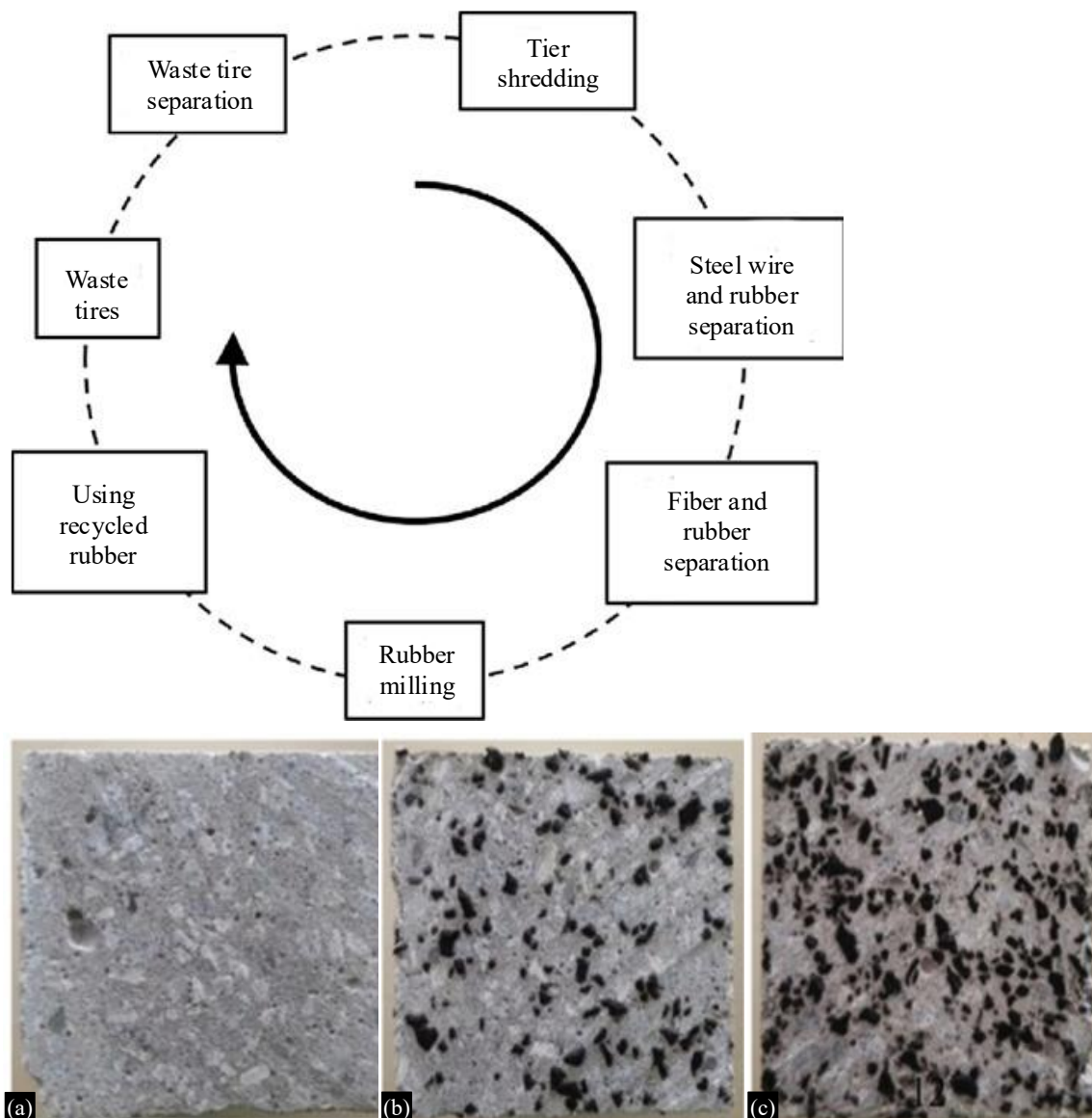
Figure 1. Internal visual inspection of the rubberized. Concrete cubes with cut-outs of 100 mm × 100 mm from the test specimens containing (a) 0%, (b) 15%, and (c) 30% rubber content.
