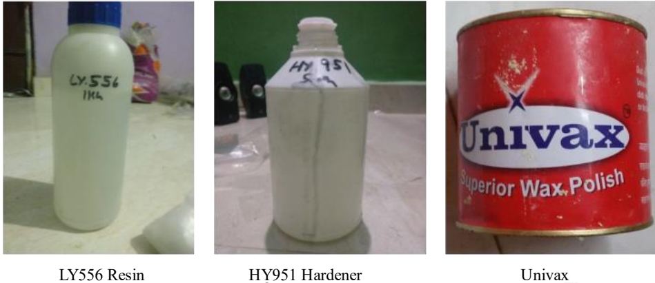
Figure 3. Resins and hardener used in fabrication.
