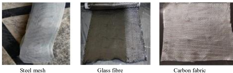
Figure 2. Steel, glass and carbon fibre.
