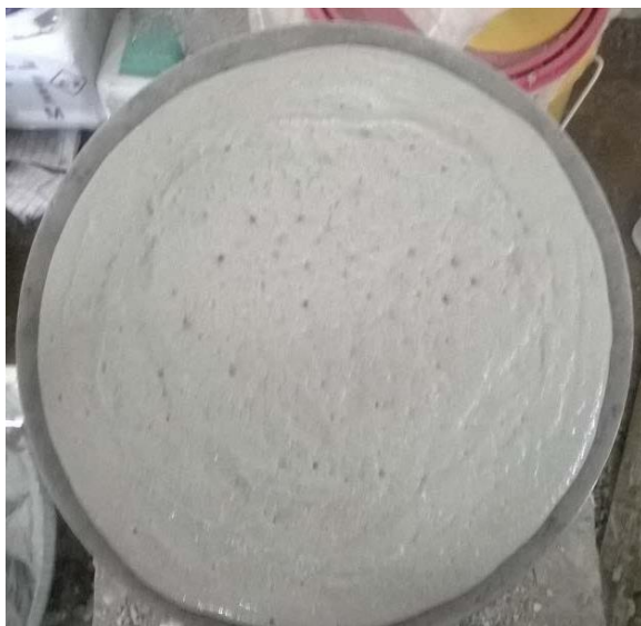
Figure 5. Flow table lean mortar mix.
