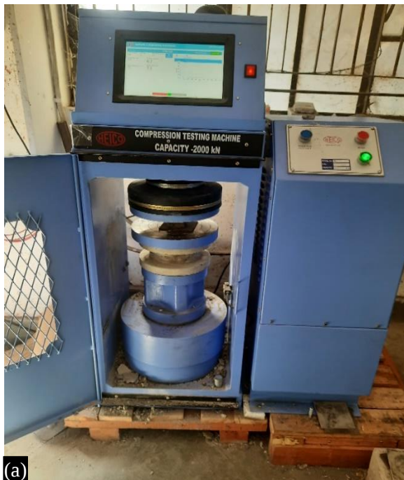
Figure 6. Compression machine (a) cube specimen and with flexural assembly (b) beam specimen.
