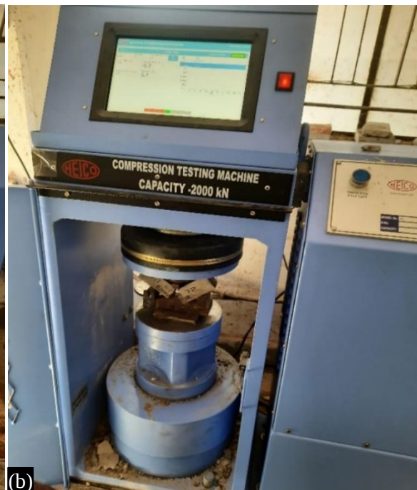
Figure 6. Compression machine (a) cube specimen and with flexural assembly (b) beam specimen.
