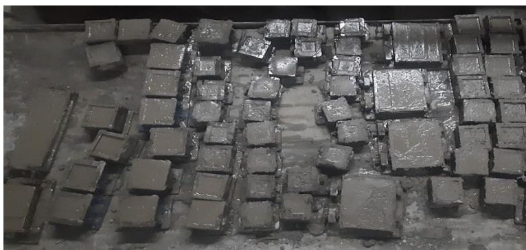
Figure 4. Casted samples of mortar.
