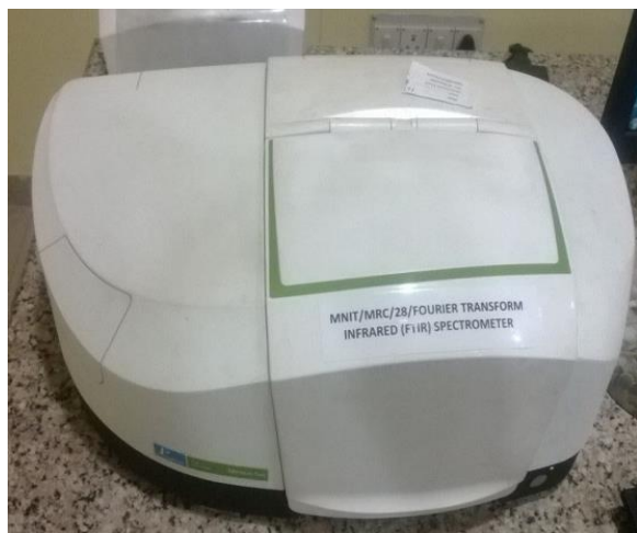
Figure 7. Fourier transform infrared spectroscopy setup
