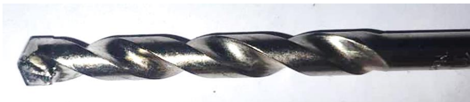
Figure 5. Sample of the Diager precision drill bit employed in the die-making operations of Koobesh Kavir Semnan Company.
