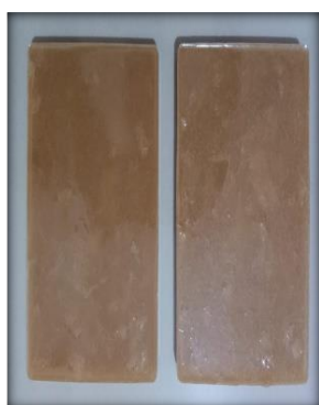
Figure 1. Fiber-reinforced composite samples (rectangular strips).
