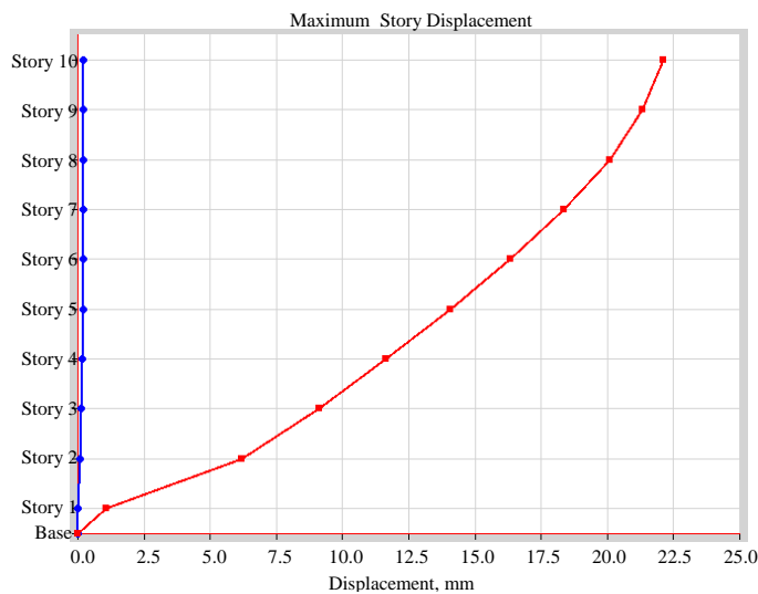
Figure 14. Displacement in Y direction: eccentric back-type bracing.
