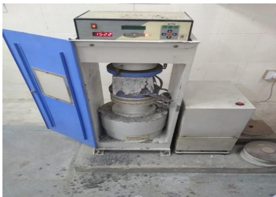
Figure 1. Compressive strength test of specimens under compression testing machine
