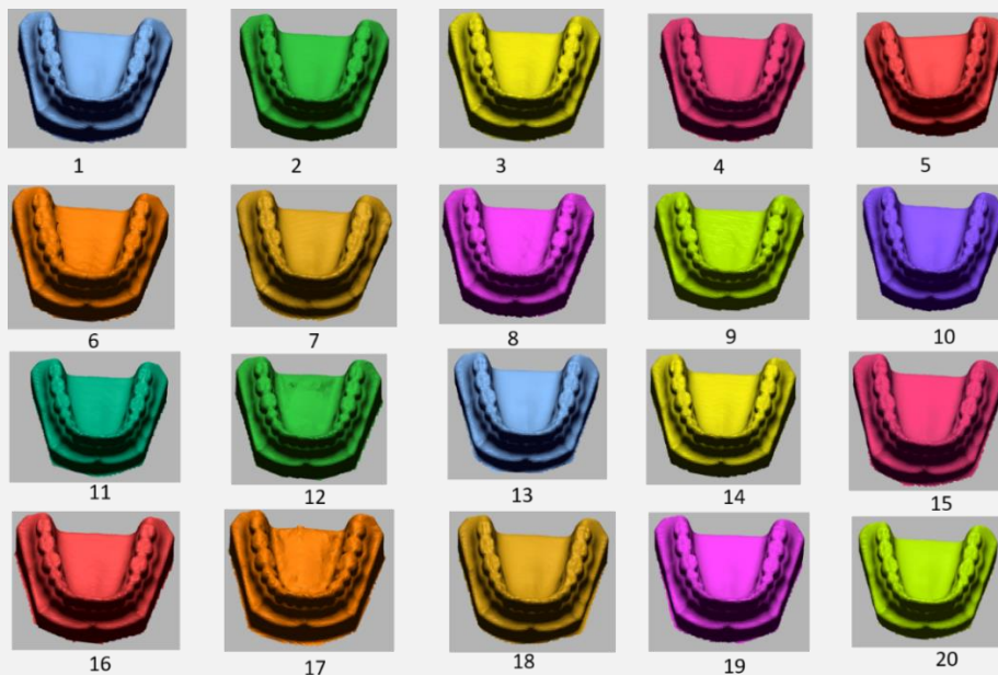
Figure 7. Twenty CAD models retrieved as per the parametric combination obtained using DoE methodology
