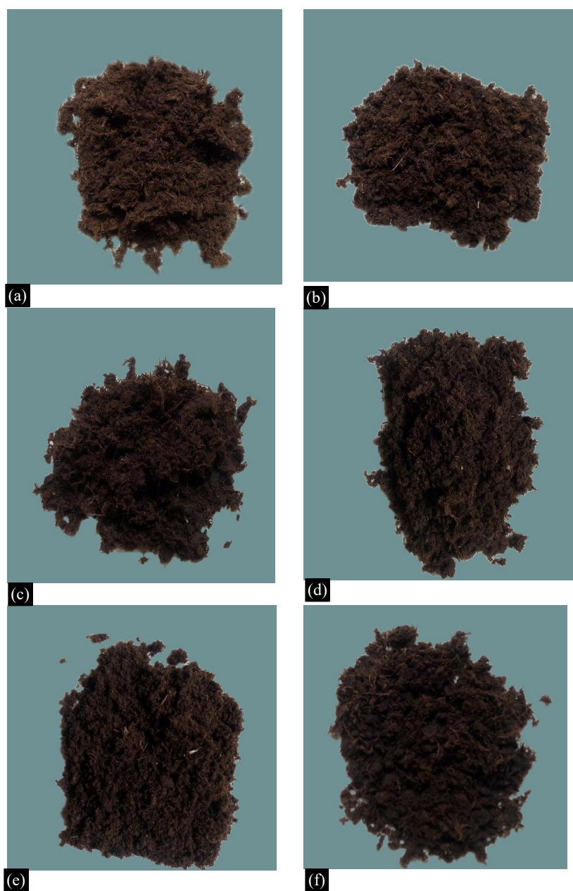
Figure 3. Digital images for steam explosion pretreated reed straws by steam flash-explosion under the steam pressure of (a) 1.0 MPa, (b) 1.2 MPa, (c) 1.4 MPa, (d) 1.6 MPa, (e) 1.8 MPa, and (f) 2.0MPa for 3 min retention time.
