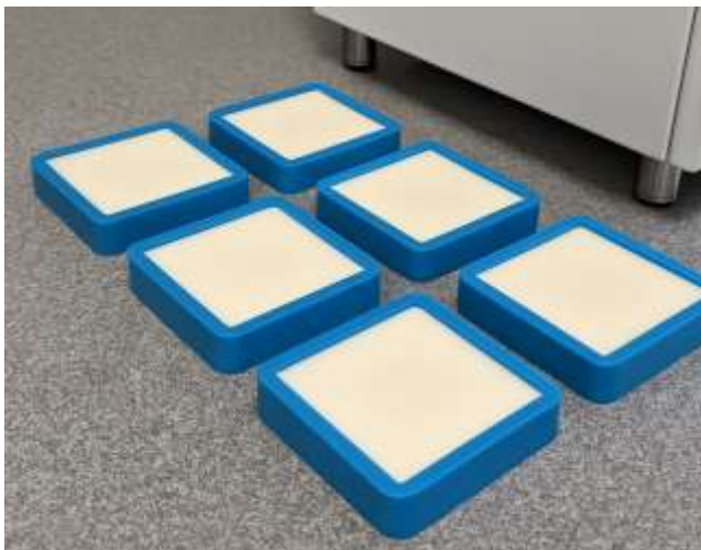
Figure 3. Casting the polymer–gel/PCM mixture into panel molds.
