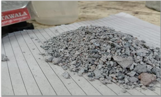
Figure 2. Obtained artificial aggregate after crushing.
