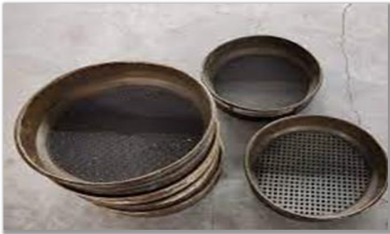
Figure 3. Indian standard test sieves set.
