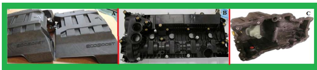
Fig. 5 (A) Engine covers, (B) cam covers and (C) oil pan manufactured by CBBP [31]
