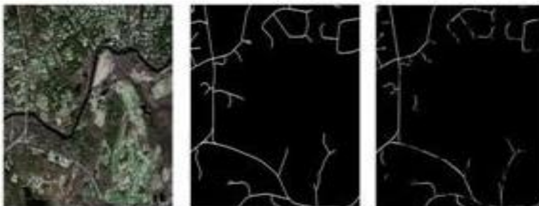
Figure 6. Example Predictions on the Test Set (a) Original image, ground truth, and predicted mask.
