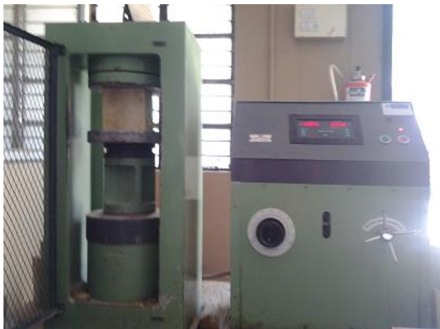
Figure 2. Compression strength test
