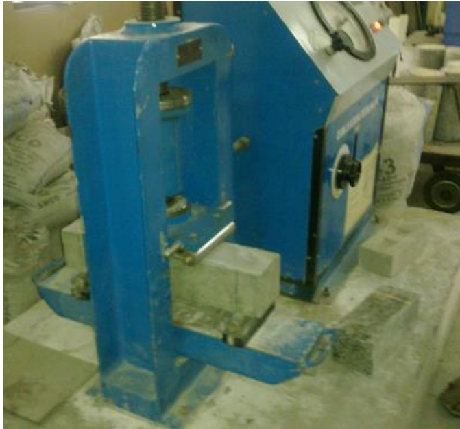
Figure 4. Flexural strength test.
