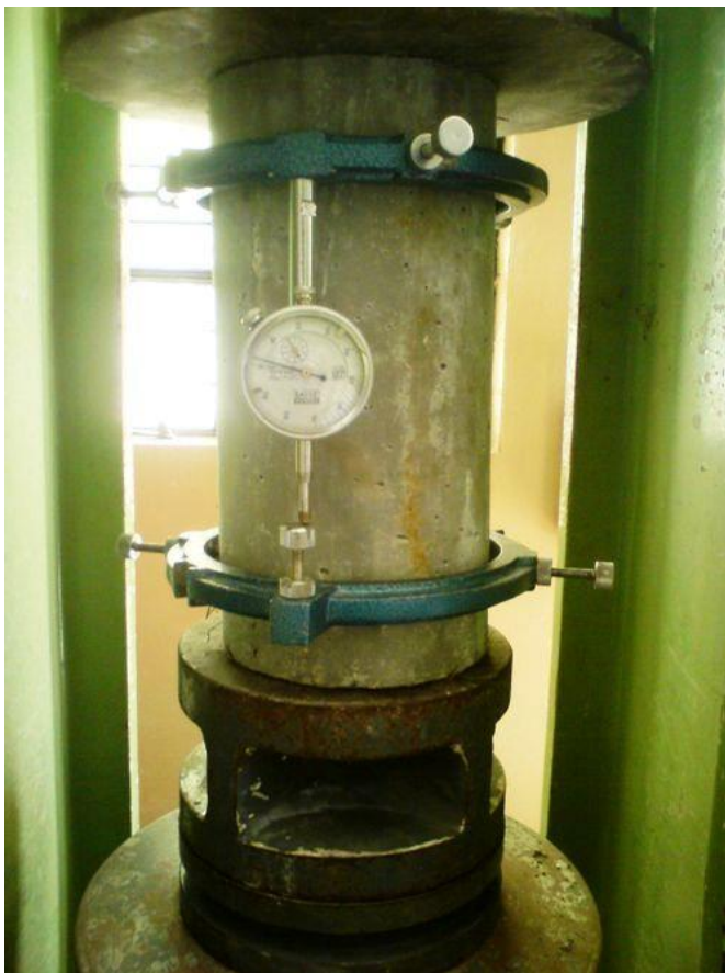
Figure 5. Test for elasticity modulus.
