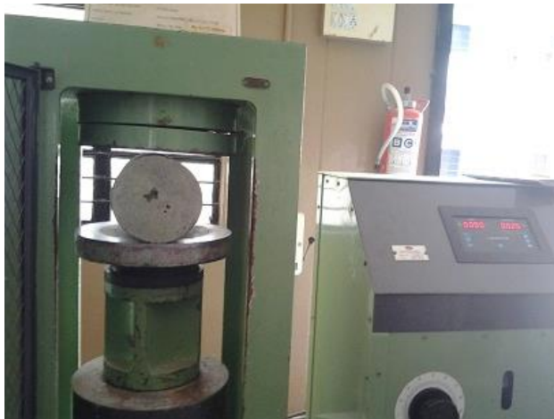
Figure 3. Split tensile strength test.
