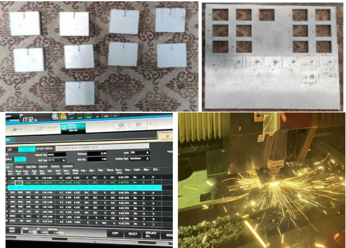
Control Panel on the CO 2 LBM Cutting of Aluminum Alloy Al [6061] and MITUTOYO SJ-210
