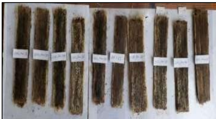
Figure 1. Nava fiber with cashew resin samples.
