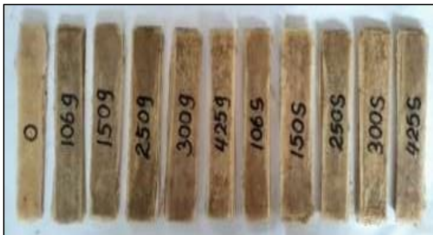
Figure 2. Nava fiber with synthetic resin samples.
