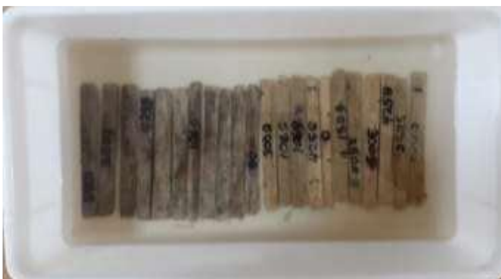
Figure 5. Water Absorption Test.
