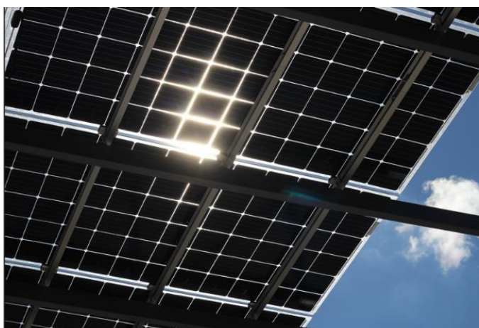
Figure 2. Bifacial solar panels for offshore applications.
