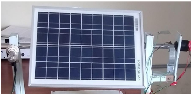
Figure 5. Sunlight intensity measurement device with solar tracking system.
